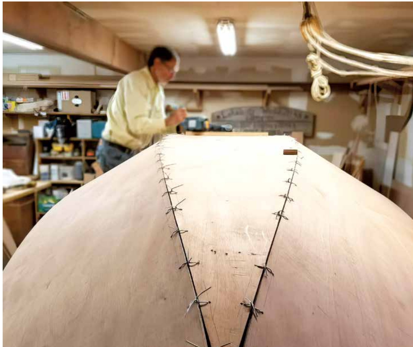
Hull panels stitched together with copper wire before gluing. Courtesy John Carlson
